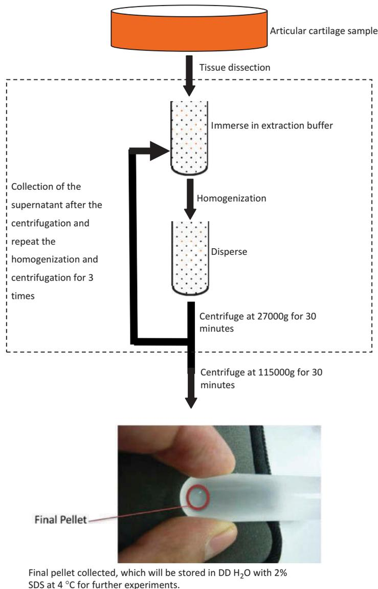
**Fig. 1.** Schematic diagram shows the extraction procedure of collagen fibrils from hyaline articular cartilages for AFM nanoindentation test.
