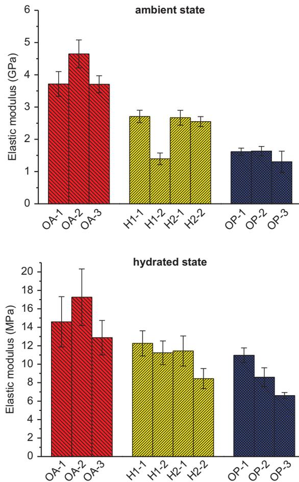
**Fig. 5.** AFM nanoindentation tests of the extracted collagen fibrils were performed under both ambient and hydrated conditions.
