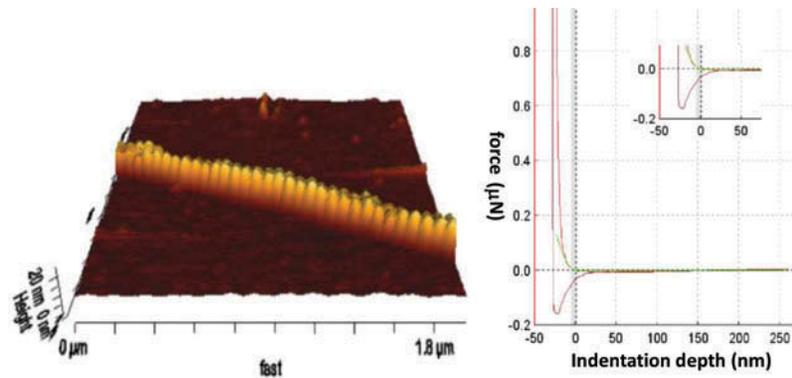
**Fig. 2.** A typical 3D image of one collagen fibril (left) and a typical  $F$ - $d$  curve of AFM nanoindentation performed (right). The green line on the right figure is the fitting curve of the experimental data with equation (1), and the fitting is good at the beginning of solid contact.
