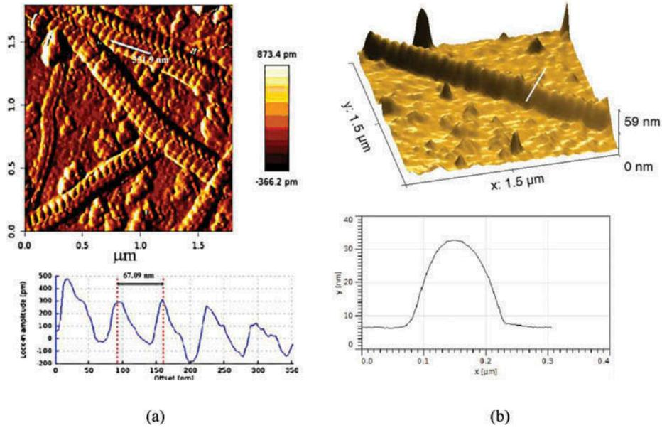
**Fig. 4.** (a) A typical AFM image showing the extracted collagen fibrils and the height profile of one collagen fibril along the longitudinal direction. The D-periodicity of the collagen fibril is about 67 nm; (b) 3D-image of a collagen fibril, the height of collagen fibrils was measured to be around 30 nm.
